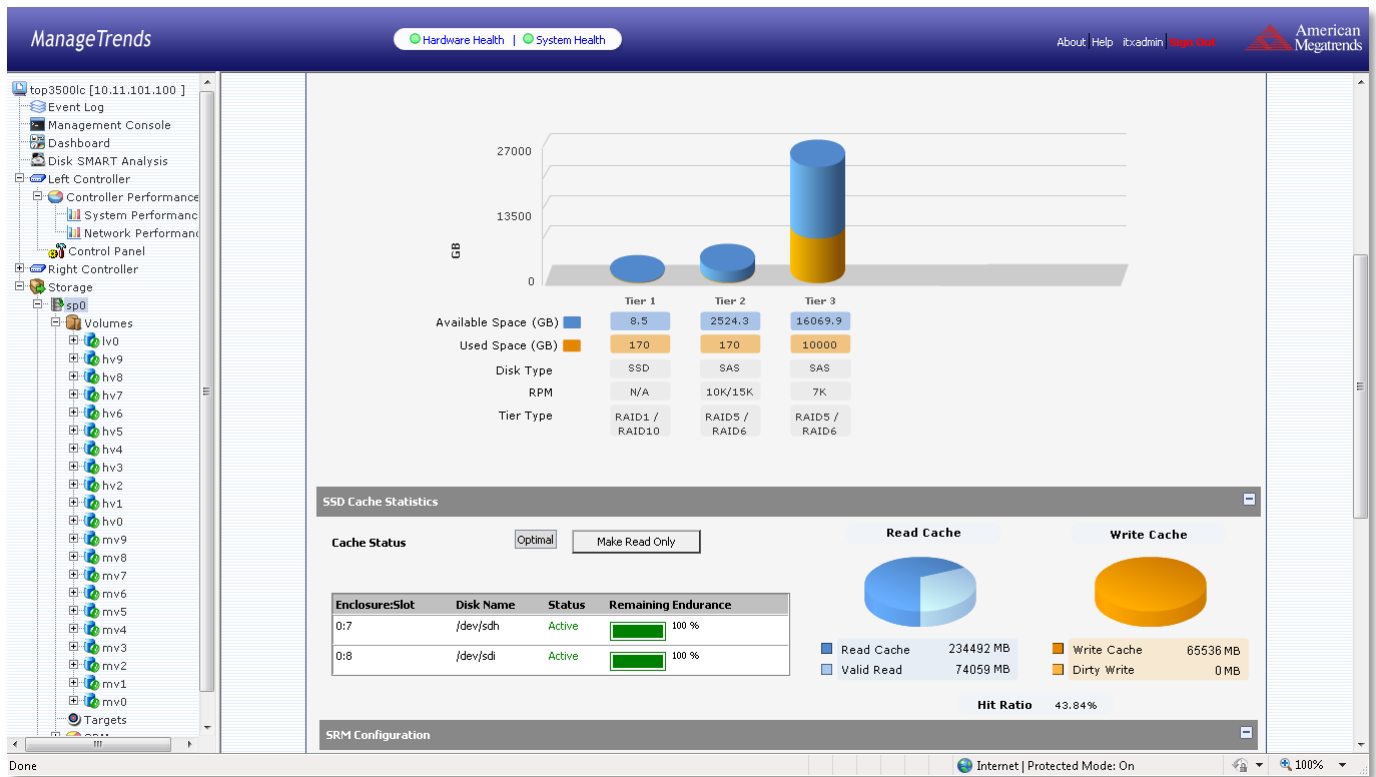
Figure 3: Our StorTrends 3500i was using 2 200GB SSDs configured into 64GB of write cache and 234GB of read cache, shown on the bottom of the image above.
